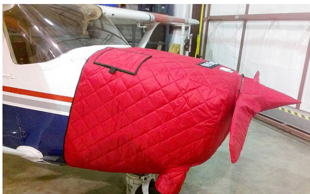
Cessna 172 Insulated Engine Cover w/ Oil Filler Door flap and Insulated Prop/Spinner Cover
