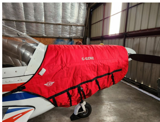
ZLIN 142C Insulated Engine Cover
