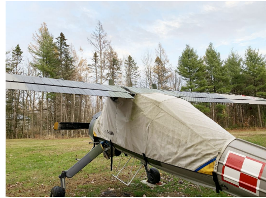
PZL Wilga Canopy Cover, Wrap-Around Type
