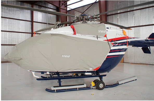
Bubble Cover w/ nose mounted radome, Upper Deck Plugs/Cover Upper Deck Plugs/Cover, extended to cover aft intake vents
