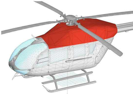
Intake/Exhaust Engine Area Cover, 3D Rendering
