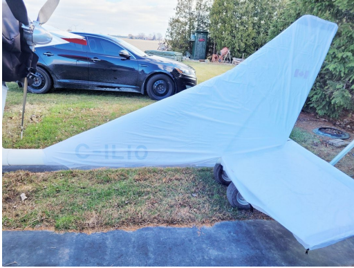
Titan Tornado Empennage Cover, test fit cover
