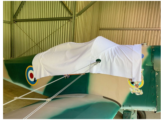
Bowers Flybaby Canopy Cover, test fit design
