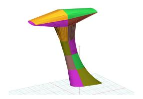
Autogyro Calidus Rotor Mast Cover, 3D model
