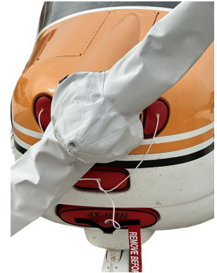
ENGINE PLUGS PREVENT BIRD NEST FOD. Piper Saratoga Engine Cowling Bird's Nest Tecnam P2002 Sierra Engine Plug Set
