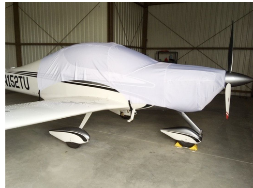
Tecnam Astore Canopy/Engine Cover, test fit cover
