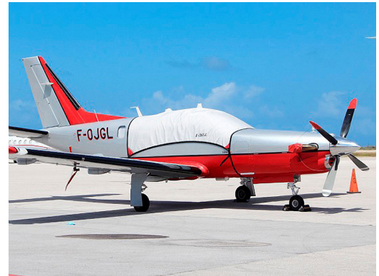
TBM Canopy Cover, Prop Tie/Exhaust Covers
