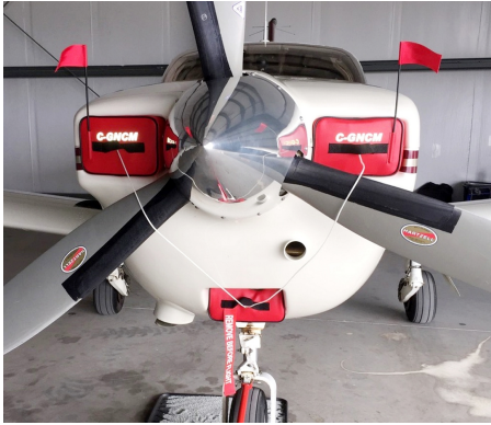
Socata TB-20 Engine Plugs, set of 3 ENGINE PLUGS PREVENT BIRD NEST FOD. Piper Saratoga Engine Cowling Bird's Nest
