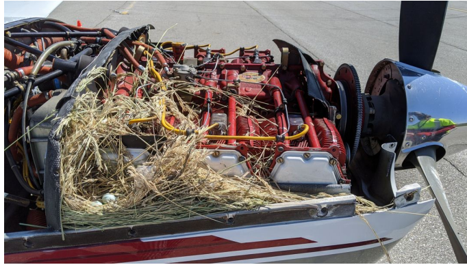
Socata TB-20 Engine Plugs, set of 3 ENGINE PLUGS PREVENT BIRD NEST FOD. Piper Saratoga Engine Cowling Bird's Nest
