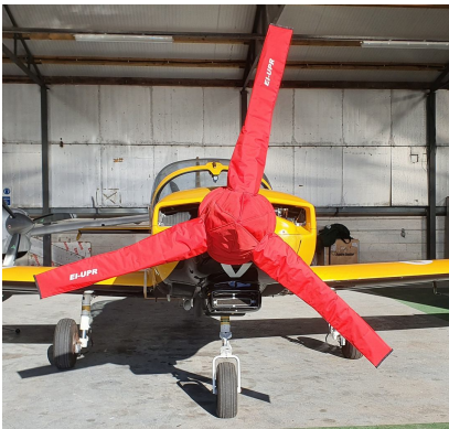
Slingsby T-67 Firefly Insulated Propellor/Spinner Cover
