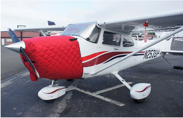
Cessna 172 Insulated Engine Cover, fully enclosed
