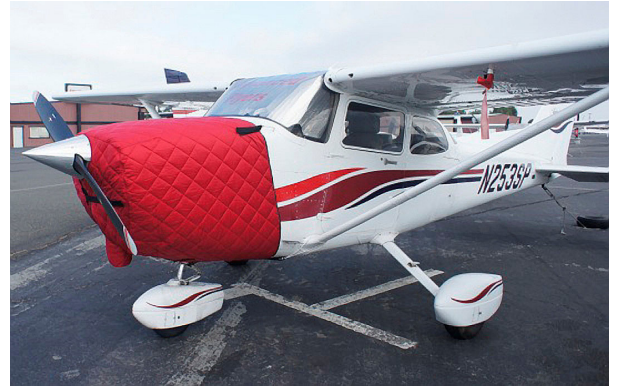
Cessna 172 Insulated Engine Cover, fully enclosed
