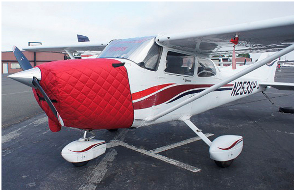
Cessna 172 Insulated Engine Cover, fully enclosed
