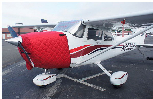
Cessna 172 Insulated Engine Cover, fully enclosed
