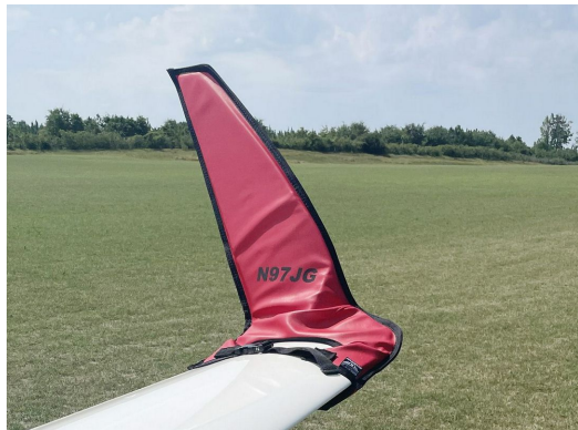
Schempp-Hirth Ventus-2B winglet/wingtip pads
