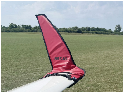
Schempp-Hirth Ventus-2B winglet/wingtip pads
