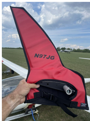
Schempp-Hirth Ventus-2B winglet/wingtip pads
