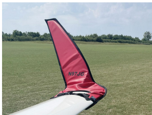
Schempp-Hirth Ventus-2B winglet/wingtip pads
