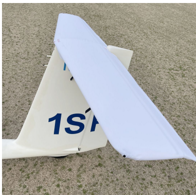
Schempp-Hirth Ventus 2B Horizontal Stabilizer Cover, test fit cover
