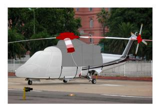
S76 Forward Fuselage, Engine, Main & Tail Rotor Hub Covers (illustration)
