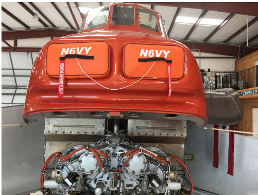
Sikorsky S58T Engine Inlet Plugs
