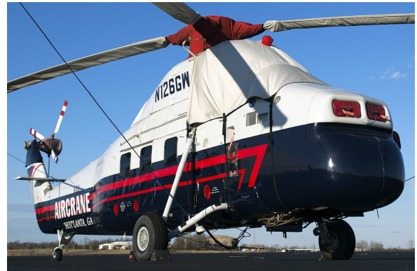
Sikorsky S58T Canopy, Rotor Hub, Blade, Tail Rotor Covers, Engine Plugs, Blade Tie-Downs
