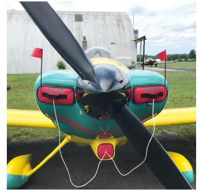
ENGINE PLUGS PREVENT BIRD NEST FOD. Piper Saratoga Engine Cowling Bird's Nest Van's Aircraft RV-4 Engine Inlet Plugs
