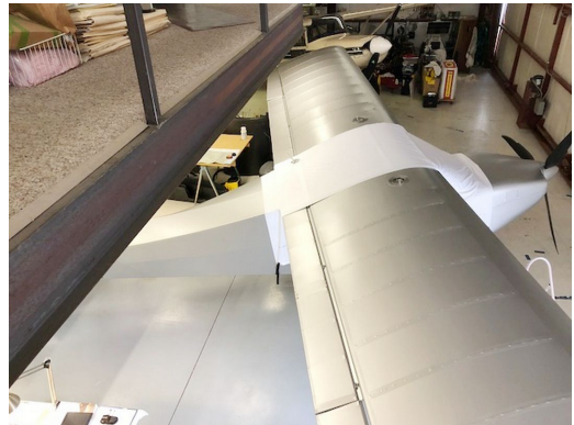
Rans S-20 Canopy Cover, test fit cover
