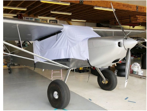
Rans S-20 Canopy Cover, test fit cover
