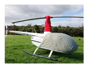
Robinson R-44 Bubble, Rotor Hub, Tail Rotor Covers, & Blade Tie-Downs
