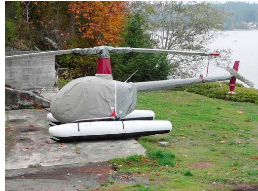
Robinson R-22 Bubble Cover (Ext. Past Rotor Hub), Engine Cover, Tailboom Cover, Blade Covers, Rotor Hub Cover, & Tail Rotor Gear Box Cover
