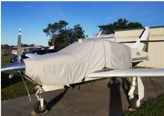
Rockwell Aero Commander 112, 114 Extended Canopy/Engine Cover
