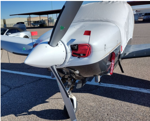
Rockwell Aero Commander 114 Canopy Cover, Engine Plugs
