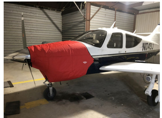
Aero Commander 112 Insulated engine cover
