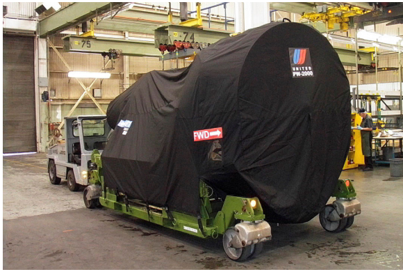
PW 2000 Series OFF-LINK ENGINE STORAGE COVER, Rain Cap PW4077 Maintenance Exhaust ShowerCap, P/N: PW-119
