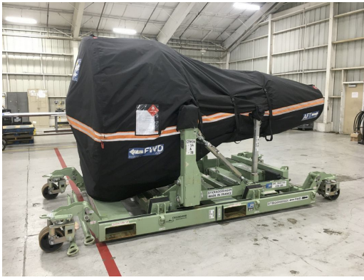
CFM56-5B Off Link Cover, fully enclosed PW JT8D Off-Link Engine Transport Cover (no nose cone, no TR's), fully enclosed
