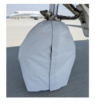
CJ1 Nose Gear Tire Cover, test fit
