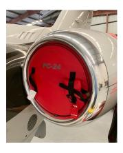
Pilatus PC-24 Engine Intake Plug
