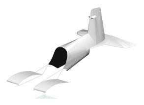
Pilatus PC-9 Empennage Cover, 3D model.
