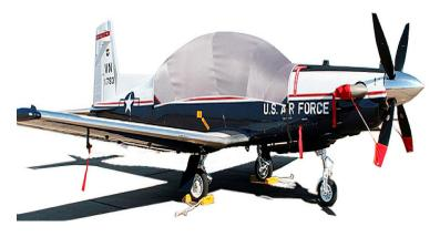
Texan II T6A Canopy Cover, Engine Inlet Plug, Prop Tie/Exhaust Covers,
