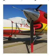
Piper PA-42 Cheyenne III Engine Plugs, Prop Ties, Cockpit Cover
