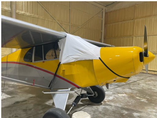
Piper J5A Windshield/Skylight Cover, test fit
