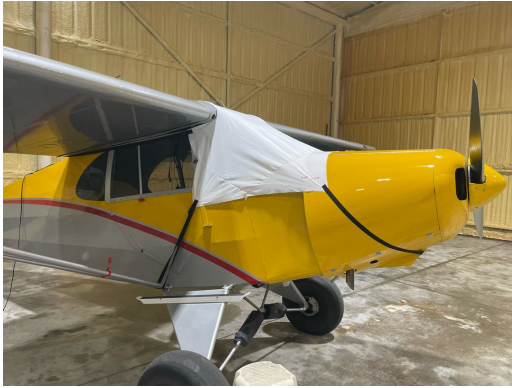
Piper J5A Windshield/Skylight Cover, test fit
