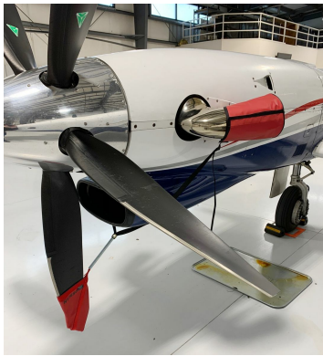
Piper PA-31T Cheyenne II Prop Tie-Downs/Exhaust Covers
