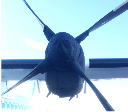
ATR-72-202 Insulated Engine & Prop Hub Covers
