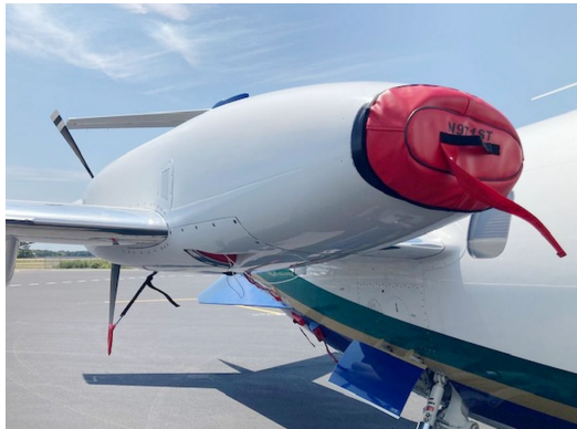
Piaggio P180 Intake Plugs with Fabric Extension
