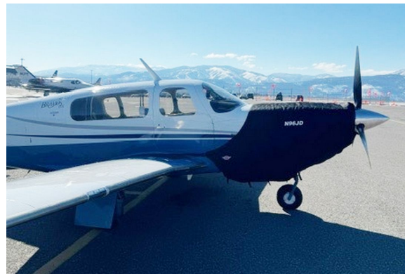
Mooney Bravo Insulated Engine Cover, Fully Enclosed
