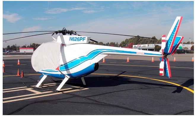
MD500C Bubble Cover with Wire Strike detail
