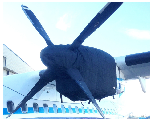
ATR-72-202 Insulated Engine & Prop Hub Covers
