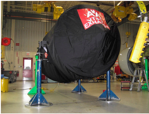
PW JT8D Off-Link Engine Transport Cover (no nose cone, no TR's), fully enclosed
