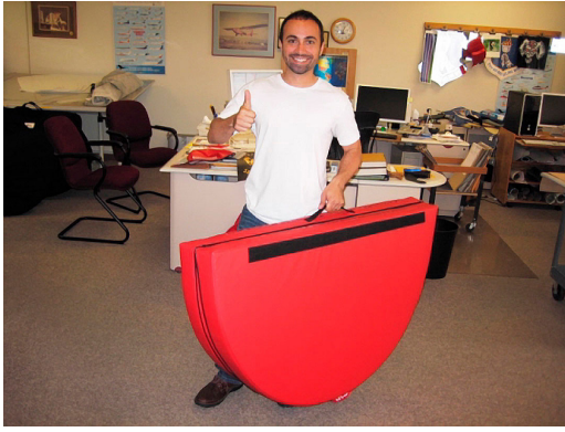
Boeing 737 FOD protection Intake Plug, folding type
