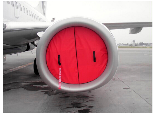
Boeing 737 Engine Intake Plug, Folding Type
