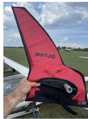
Schempp-Hirth Ventus-2B winglet/wingtip pads
