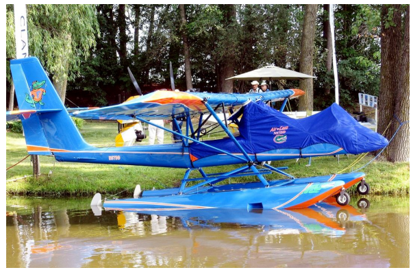
CANOPY/NOSE/BAGGAGE AREA COVER, with aft flat windshield
