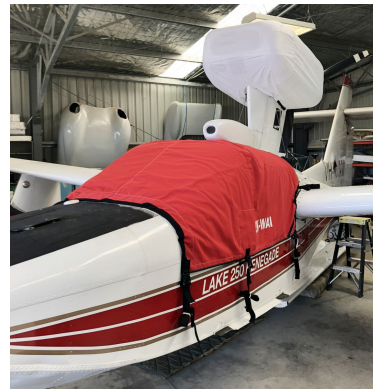
Lake LA250 Renegade Cockpit Cover, Engine Cover (test fit)
