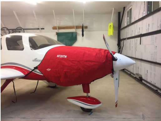
Lancair ES Insulated Engine Cover, Fully Enclosed
