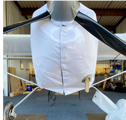
Kitfox Extended Canopy/Engine Cover, test fit cover
