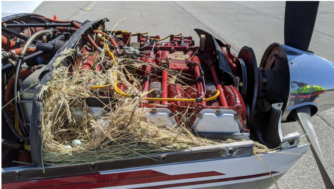
ENGINE PLUGS PREVENT BIRD NEST FOD. Piper Saratoga Engine Cowling Bird's Nest Preceptor STOL King Engine Plugs
