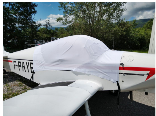
Jodel D113V Canopy Cover, test fit cover
