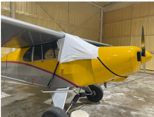
Piper J5A Windshield/Skylight Cover, test fit
