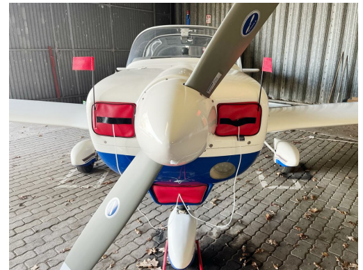
Grob 115 Engine Inlet Plugs, Incl. Carb. Inlet Plug
