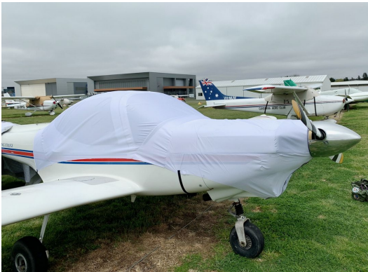
Grob 115 Canopy/Engine Cover, test fit cover
