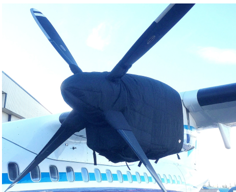
ATR-72-202 Insulated Engine & Prop Hub Covers
