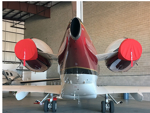
Canadair Challenger 300 Intake/Exhaust Covers, 3-Strap Type
